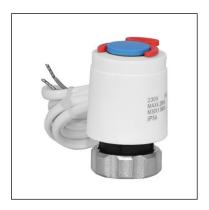
The A24NC normally closed thermoelectric actuator is designed for controlling small thermostatic valves or manifolds in heating and cooling systems. It can be controlled with an on/off controller or switch.
